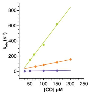
**Figure 3.** Apparent rates  $k_{\text{obs}}$  for CO binding to ferrous Mt-trHbN. Curves for wild type (green), VG8F (orange) and VG8W (violet) mutants as a function of CO concentration in stopped flow measurements are shown. The time courses are measured at different CO concentrations ranging from 10 to 200  $\mu\text{M}$  (after mixing). Continuous line corresponds to linear fit of  $k_{\text{obs}}$  rates.
