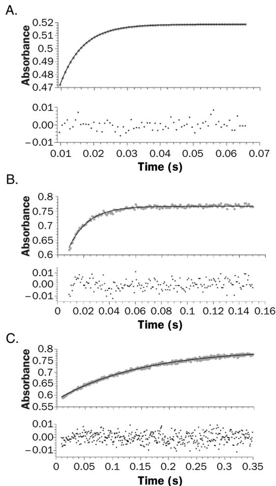
**Figure 2.** Stopped-flow time course for the reaction of reduced 5  $\mu\text{M}$  wild type (A), VG8F (B), and VG8W (C) mutants in 100 mM phosphate buffer at pH 7. The reaction was monitored at 423 nm (grey dots) and the line shows the best first order fit.
